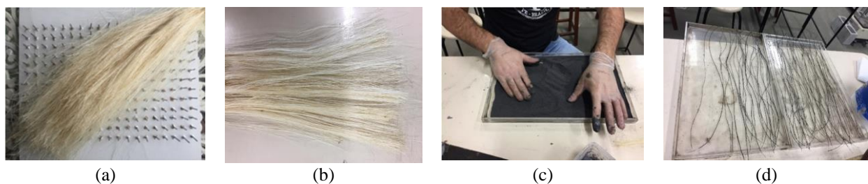
Figure 1 – Surface treatment applied to the sisal fibers: (a) Untangling process, (b) fibers " in natura ", (c) adhesion of ferromagnetic residue to fibers and (d) treated fibers before cutting.
